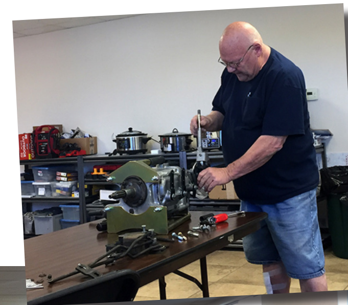
Gary Steffens demonstrates how to adjust shifting linkage on C1 and C2 transmissions
