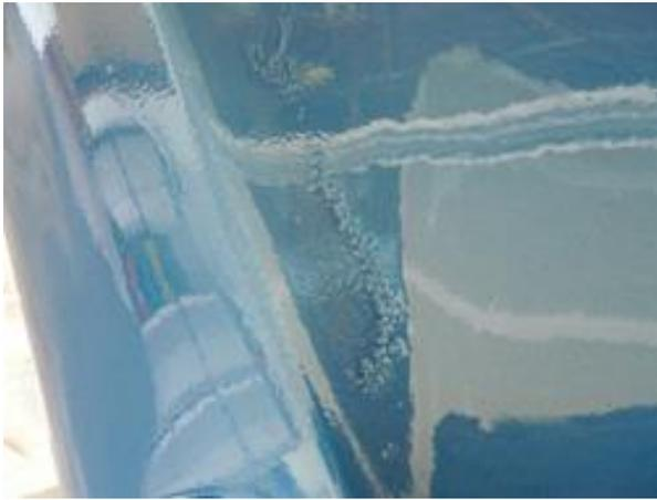
What had happened was residual brake fluid was still absorbed in the raw fiber glass and out gassed into the paint . So, I stripped back the contaminated area to the raw fiberglass. Once the fiber glass was stripped I soaked the under and top sides of the fender with Acetone, finishing with lacquer thinner. I let the Corvette sit for a couple of weeks in the heat.
