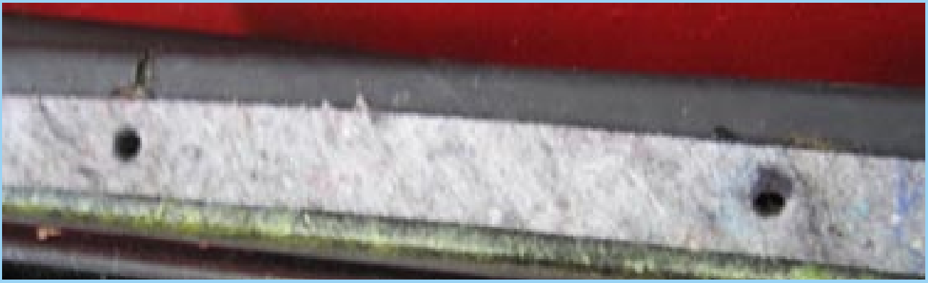
Metal strip holding rubber W/S to convertible frame
