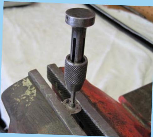
Cleaning threads on the barrel nuts
