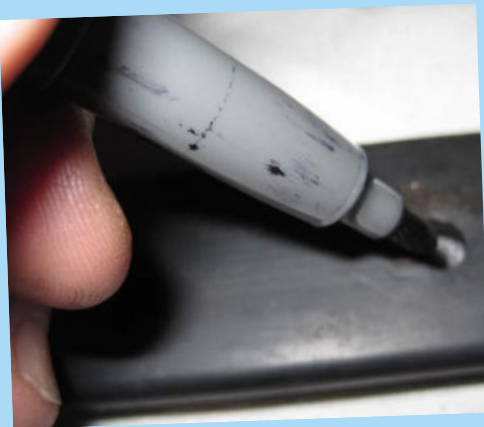
Marking W/S felt with rubber W/S as guide for hole punching
