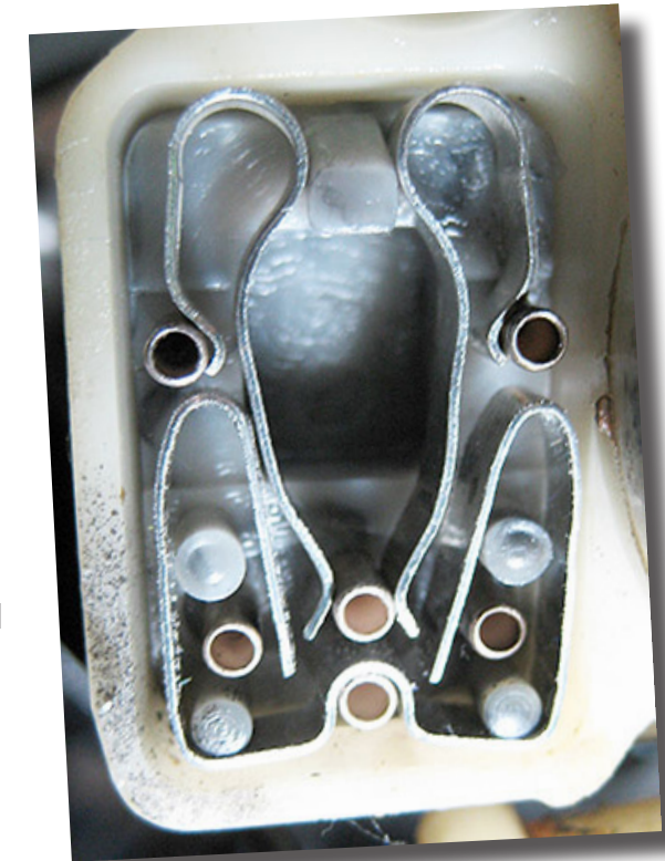
Photo 8 – Incorrect Spring Material
