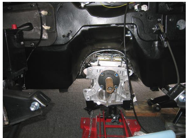
Place the TK0600 on a transmission jack and do a placement and alignment checkout, since the TK0600 is taller from top to bottom than the Muncie, there will be very little distance between the top of the TK0600 and the bottom of the shifter plate.
